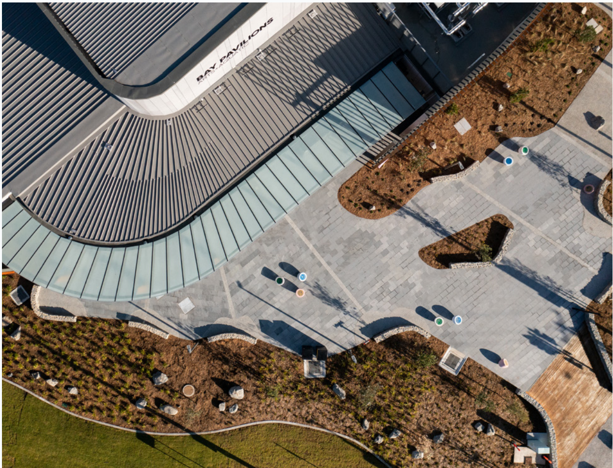
Figure 15. The NBRSLandscape team incorporated endemic native vegetation into the landscape design to minimise water use, improve drought tolerance and support local biodiversity. (Image: Alexander Mayes Photography)
