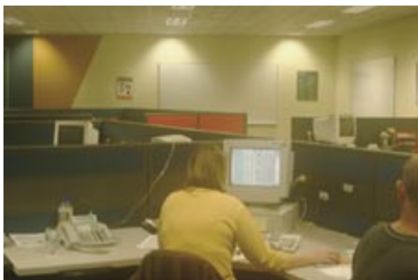
Figure 3. The screen on the workstation is far too dark so that the luminance contrast between the screen and the VDU is excessive. Although the back wall is being lit the contrast between the bright and dark sections of wall is too great and the lighting seems to accentuate the darkness rather than making the space look lighter.
