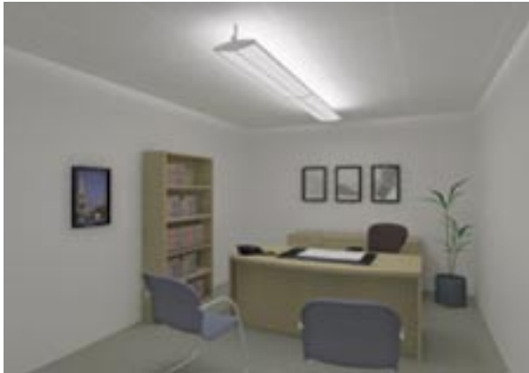
Figure 9. A detailed rendering from a flux transfer program. Note that although the view is detailed the shadows are soft and there are no reflections in the shiny surfaces 2 .
