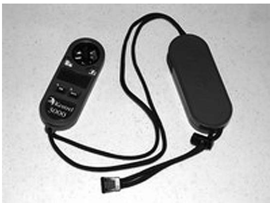
Figure 9. A hand-held digital averaging anemometer for on-site measurements
