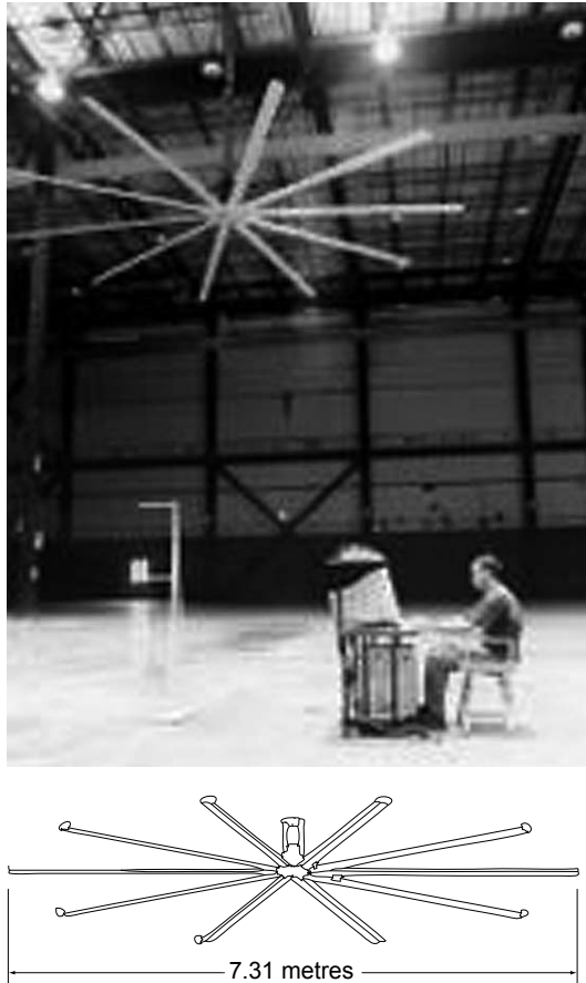
Figure 3. Measuring airflow from a 7.3M diameter hvls industrial ceiling fan
