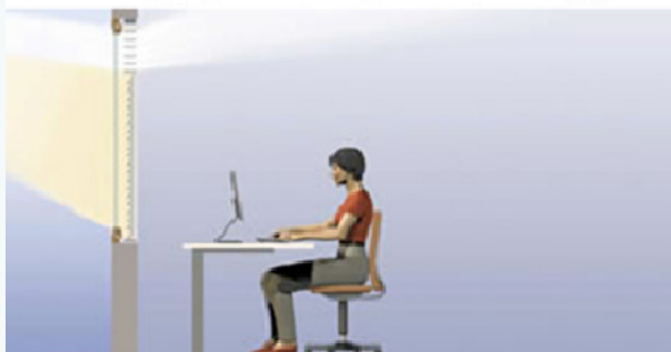
Direct light deflected, top slats adjusted to reflect on to ceiling, allowing natural light with no glare.
