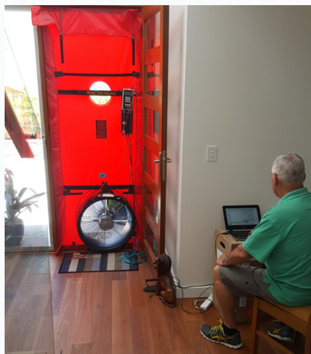
Figure 5. Installation of the fan for a blower door test. The fan is used to induce pressure in the building in two modes – pressurisation, or blowing air in, and depressurisation, or pulling air out. (Image: Blower Door Services n.d.)
