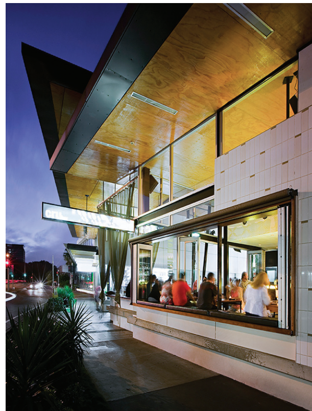
Retractable windows assist with the natural ventilation of the market and allow patrons to enjoy the subtropical climate. (Image: CF Jones, 2010)
