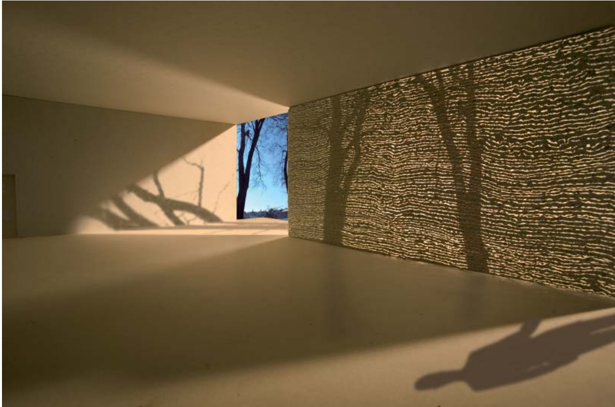
Figure 4: Light transmitting concrete (Photo: Aron Losonczy, www.litracon.hu Litracon)
