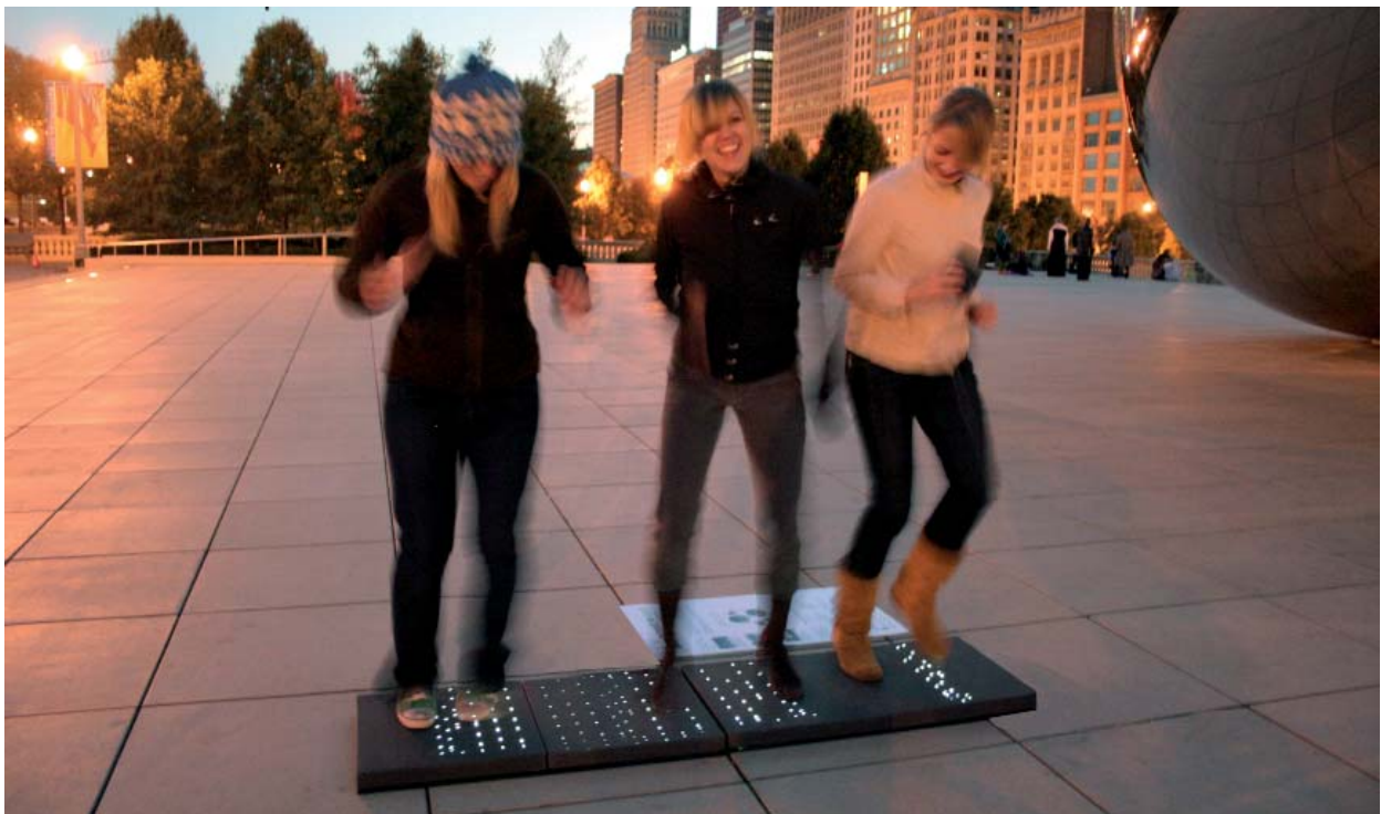
Figure 1: Energy harvesting flooring that converts kinetic energy into electricity (Source: Courtesy of POWERleap, Photo: 2007)
